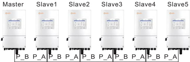
Figure 3.24 Parallel Terminal Connection
