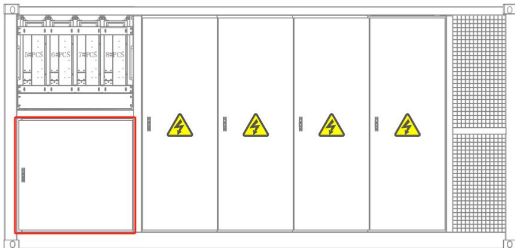
Figure 6-3 The door of primary distribution box(Left view from back of the container)
