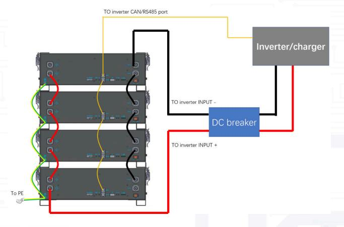
Type 2: Maximum continuous current 200A, maximum energy storage output power 10kW.
