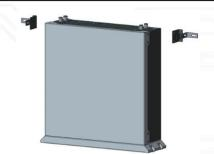
VIII. Remove hang ear from the battery, and drill holes in the wall for the M6 expansion bolt. The drilling depth should be at least 50 mm, insert the bolt.
