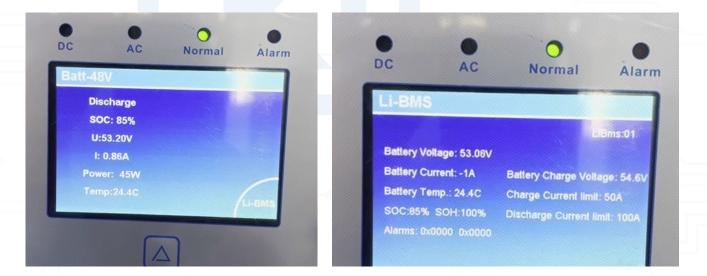
5 Confirm all the parameters and then finish other settings (TOU, Zero export etc.) on the inverter according to the inverter manual. 6 If parameters are set correct, you are ready to use the system.
