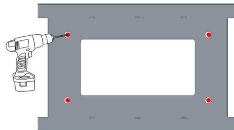
VI. Fix the wall mounting widget and the decorative panel with the battery using the combination screw
