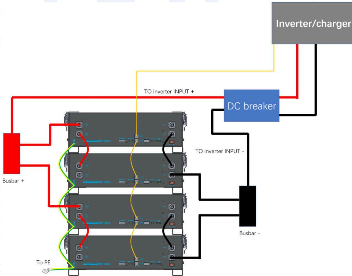
**Type 3: Maximum continuous current 400A, maximum energy storage output power 20kW.**
