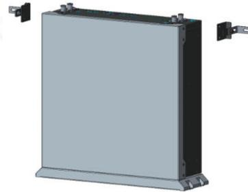
VIII. Remove hang ear from the battery, and drill holes in the wall for the M6 expansion bolt. The drilling depth should be at least 50 mm, insert the bolt.
