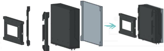
VII. Lift the battery up and put the hook into the bracket hanging hole, fix the widget with the bracket via the combination screw and tighten it using a screwdriver
